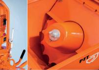
The feed tray nut can be easily opened even after a long period of operation since the thread is protected from dust.
