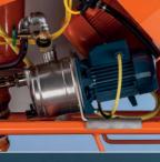
Improved water outlet by tilting the pump and optimum frost protection since the residual water can be drained completely.
